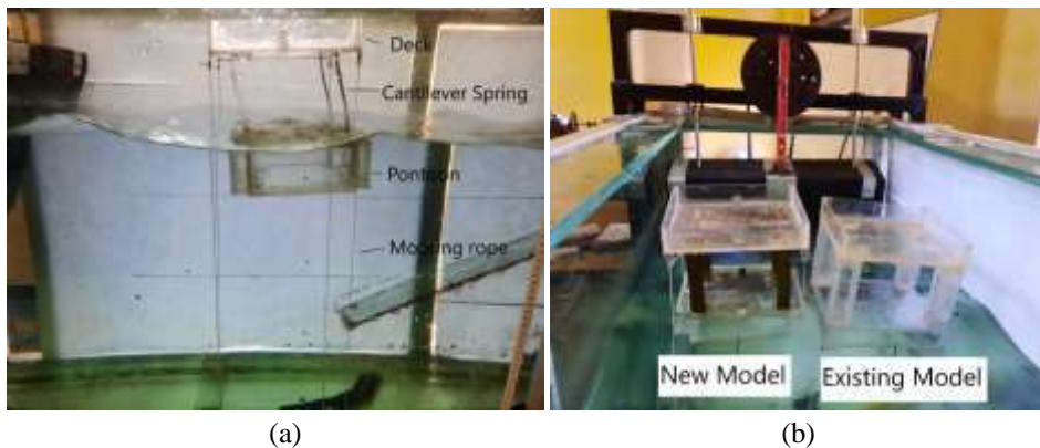
Figure 4. (a) Water waves as a medium, and (b) The new model (TLP 2-DOF) and the existing model.
