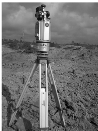
Gambar 3. Alat Terrestrial Laser Scanner
