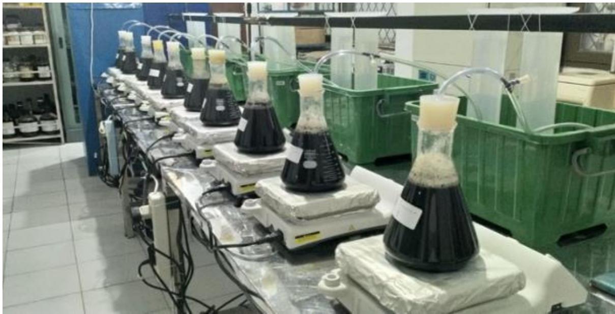
Figure 1. Digester arrangement to evaluate cassava pulp addition and delaying time during biogas production using tapioca wastewater.
