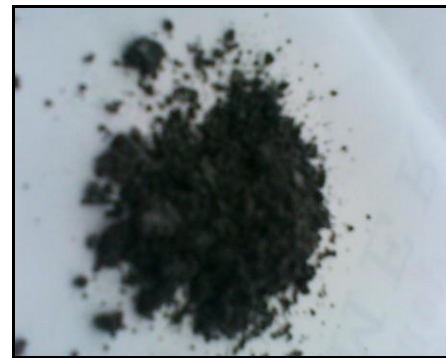
Fig. 4. Organic clay material (illite+naphthalen)
