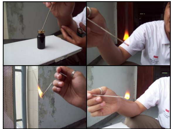
Fig. 13. Combustion test on the fluid the result of organic clay and organic carbonate material
