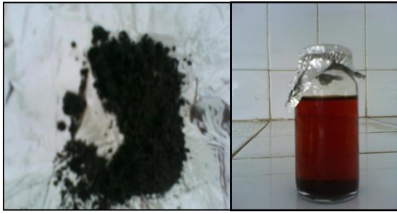
Fig. 5. The heating of organic clay at T=300^{\circ}\text{C}
