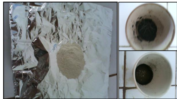
Fig. 10. The heating of organic carbonate material at temperature of 900^{\circ}\text{C} and 1000^{\circ}\text{C}
