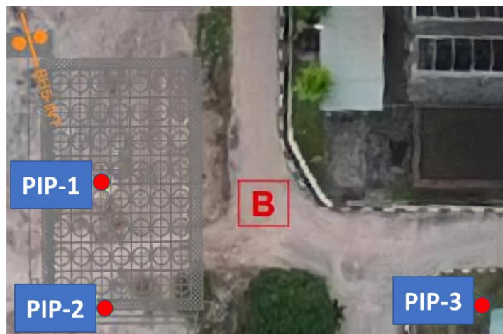
Figure 3. Location plan of GPR, PIP 1, 2, and 3 measurement points. The gray schematic at the PIP 1 and the PIP 2 is the former building site plan that contains spun pile features beneath the surface.
