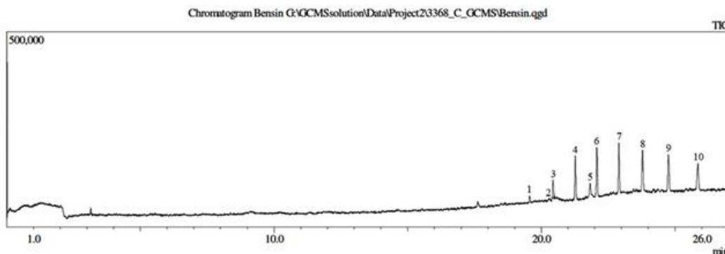
Figure 4. GC-MS Chromatogram Profile of Oil#3 from Pyrolysis of Plastic Waste. Peaks: (1) n-Pentadecane; (2) Cis-1,3-Dimethoxycyclopentane; (3) n-Eicosane; (4) n-Heptadecane; (5) Diethylphthalate; (6) n-Tricosane; (7) n-Pentacosane; (8) n-Hexadecane; (9) n-Hexatriacontane; (10) n-Octacosane
