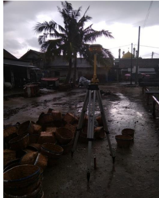
Figure 3. Ground Control Point Measurement
