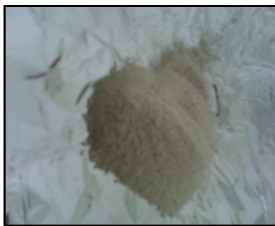
Fig. 7. The heating of organic clay at T=1000^{\circ}\text{C}
