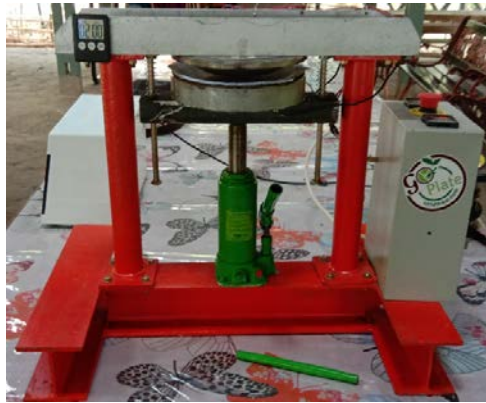
Fig. 4. Photo of the Teak Leaf Plate Molding Machine
