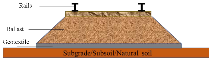
Figure 11: Use of Geotextiles on Railways
