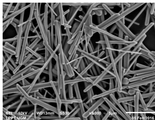
Figure 5. SEM images of silver nanowires by using PVA and PVP for molar ratio [PVA:PVP] of 3:7.
