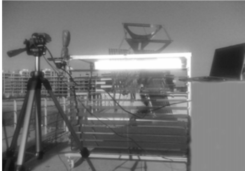
Fig. 3. Photograph of the experimental set-up. It can be seen on the right the lap top controlling the CCD camera (on the left). In front of the camera, the image shows the concentrator focusing incoming radiation towards the lambertian surface.
