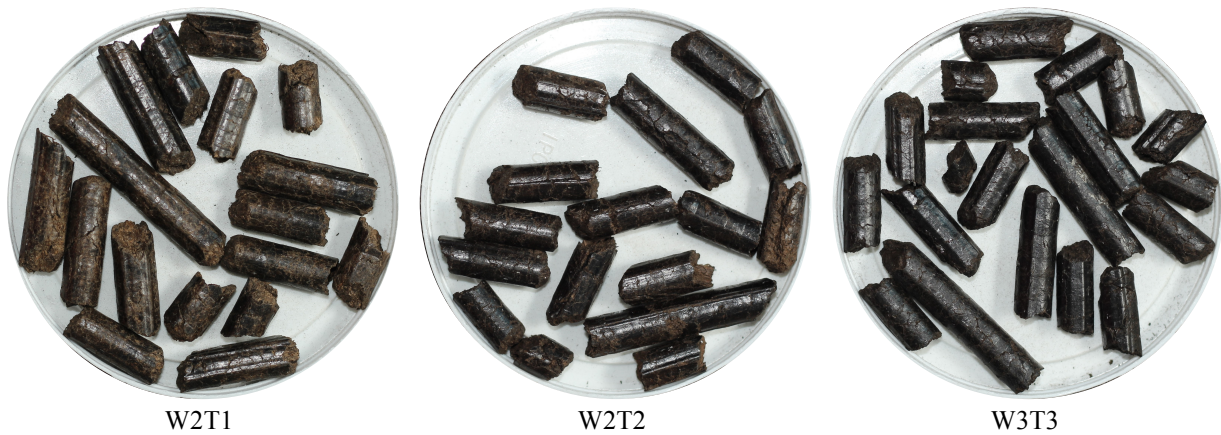
Figure 3. Example of torrefied pellets with torrefaction duration of 10 min (T1), 20 min (T2), and 10 min (T3)
