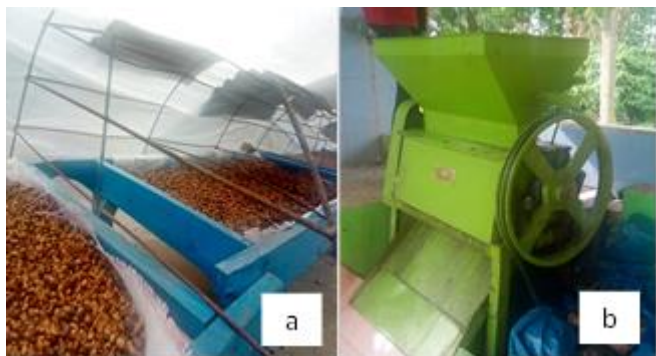
Figure IV. Postharvest treatment: a) sun dryer, b) pulping machine
