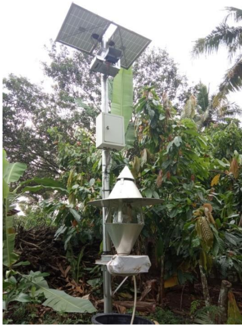
Figure 4. The automatic insect trap in cacao plantation
