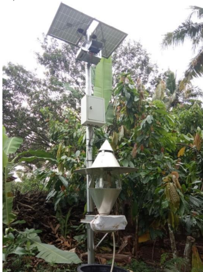
Figure 4. The automatic insect trap in cacao plantation
