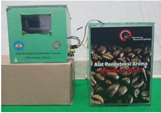
Gambar 5. Ruang Kendali dan chamber sensor electronic nose
