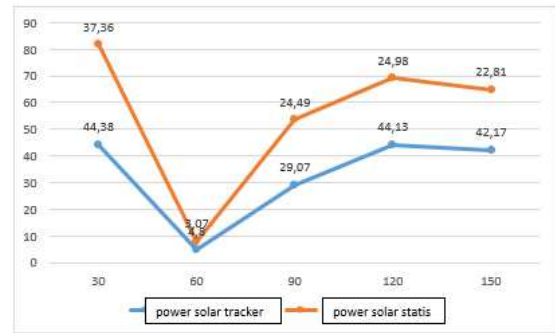
Figure 13. Graph of the tilt angle to the power generated by the solar panel
