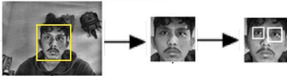
FIGURE 7. The eye detection process using the Viola Jones method.
