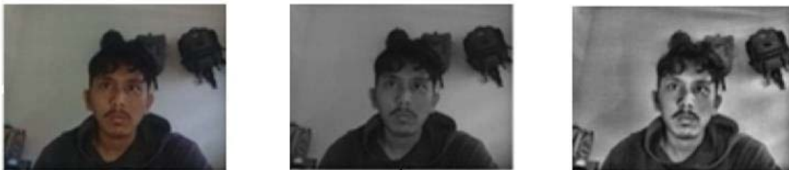
FIGURE 3. An example of an image frame captured by a camera. (a) Color image, (b) Grayscale image, and (c) Histogram equalization image.
