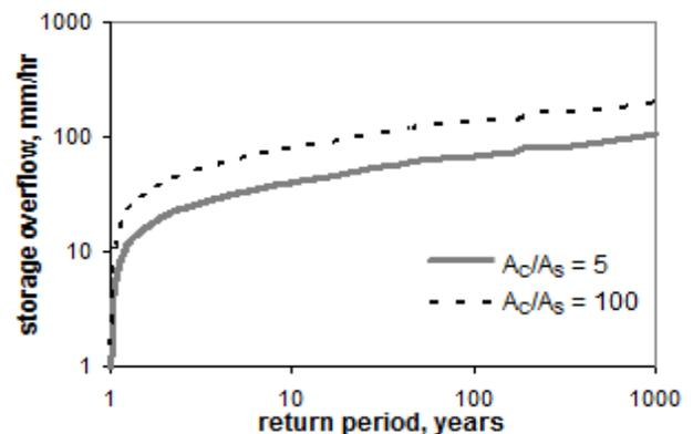
**Figure 2.** Flood Frequency Curve of Storage Overflow
