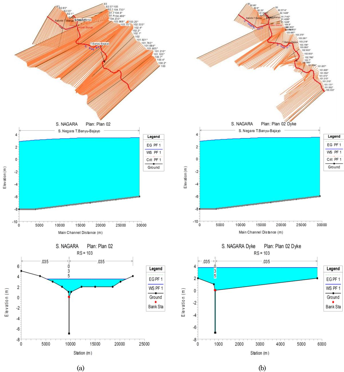
**Figure 4.** River Geometries (top figures), Water Surface for Long Profiles (middle figures) and Cross Sections (bottom figures) in the Simulation at Existing Condition or without Dyke (a) and with Dyke (b)
