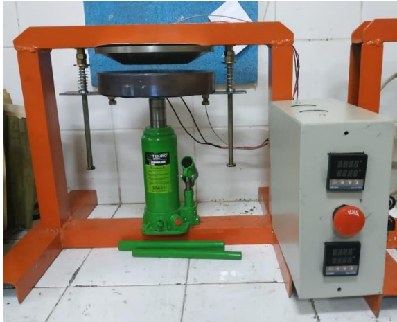
Figure 3. Leaf Plate Molding Machine
