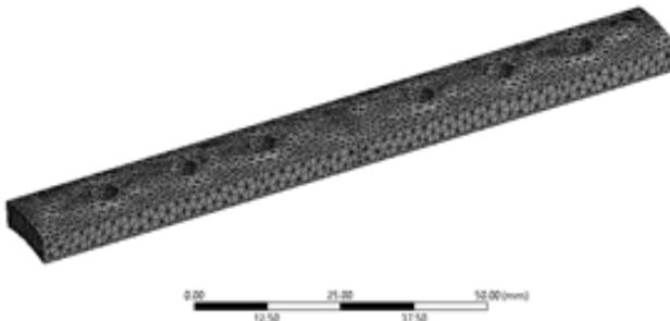
Gambar 4. Geometri elemen meshing tetrahedron 6 lubang
