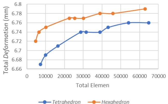
Gambar 12. Total deformation elemen hexahedron dan tetrahedron 10 lubang
