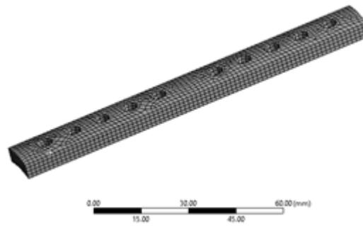
Gambar 7. Geometri elemen meshing hexahedron 10 lubang
