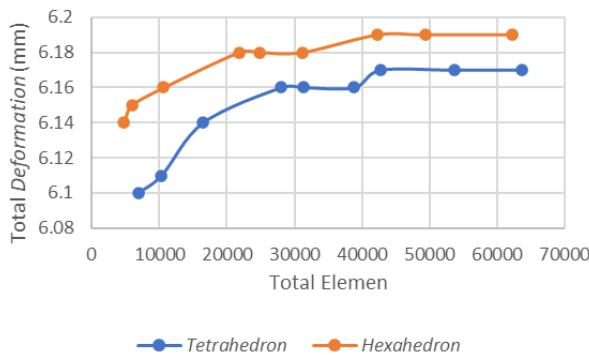
Gambar 13. Total deformation elemen hexahedron dan tetrahedron 6 lubang
