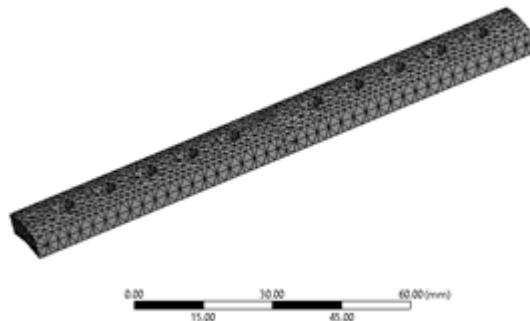
Gambar 6. Geometri elemen meshing tetrahedron 10 lubang
