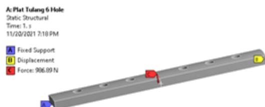
Gambar 9. Boundary conditions 6 lubang
