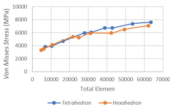
Gambar 10. Von misses stress meshing tetrahedron dan hexahedron 10 lubang
