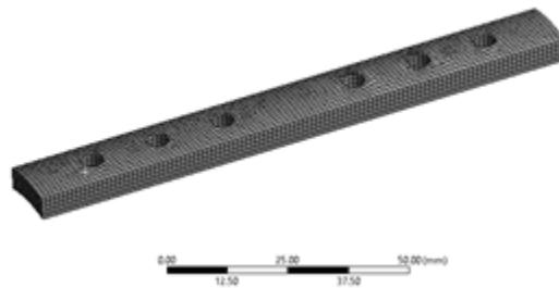
Gambar 5. Geometri elemen meshing hexahedron 6 lubang
