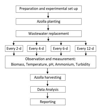
Fig. 2 Flow chart for the whole experiment
