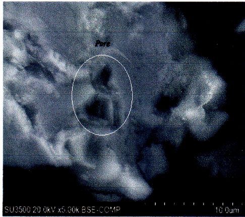
b) Figure 5. a) SEM from recycle refractory with kaolin clay addition with sintering at 1200 °C for 10 hours. b) SEM from kiln used refractory.
