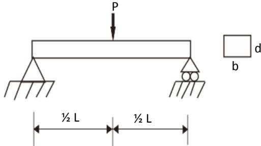
Gambar 8. *Three point bending*
