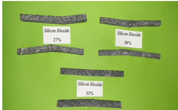
Figure 3. Deformation specimens after testing
