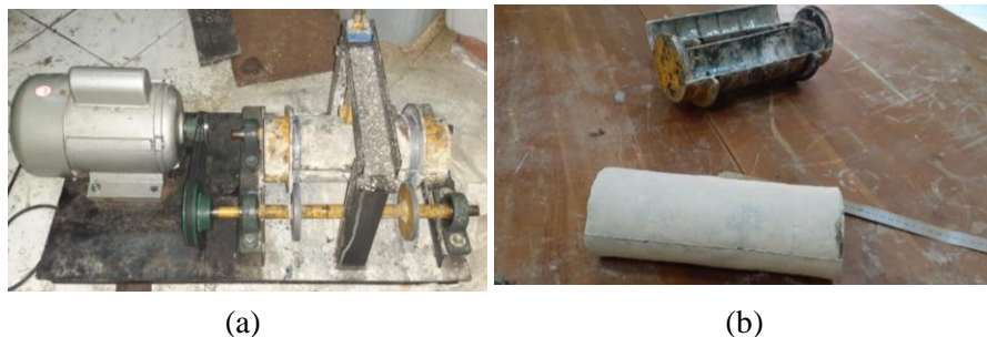
Figure 1. (a) Centrifugal machine testing, (b) The molded pipe
