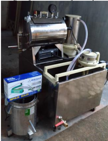
Gambar 2. Alat penggorengan vakum ( vacuum frying )
