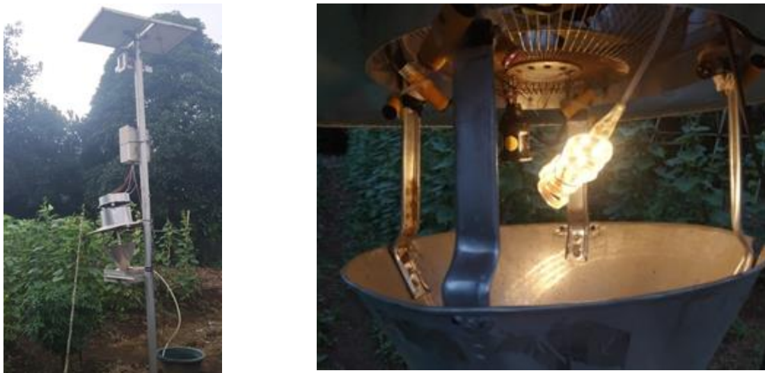
Figure 3. (a) Automatic trap and Cucumbers plant (b) Yellow LED light on automatic trap
