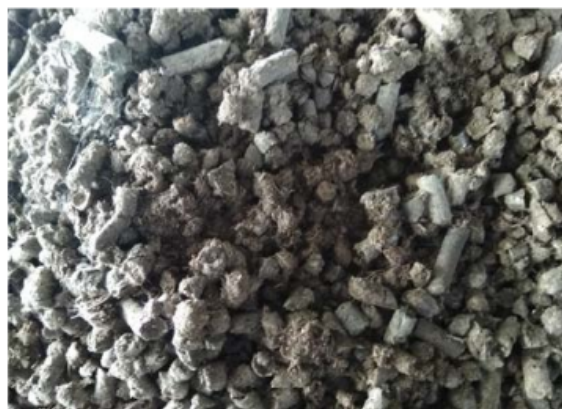
Fig. 3. Rotten OPEFB pellets stored improperly in open space
