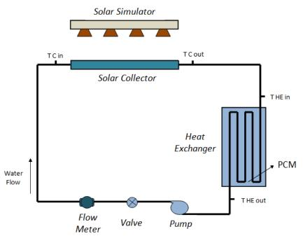
Fig. 1. The scheme of water heating test equipment using PCM
