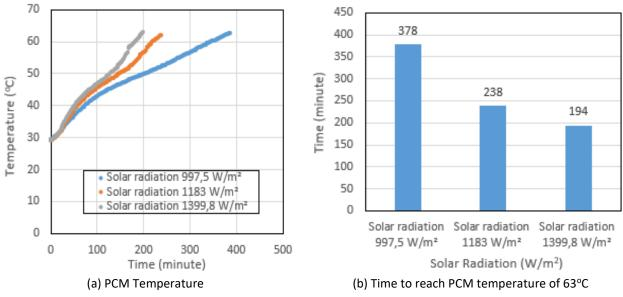
Fig. 4. Effect of solar radiation on the average PCM temperature for a water flow rate of 2 lpm
