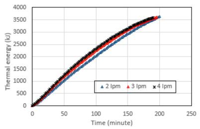
Fig. 5. Thermal energy released by water in PCM heating process in HE for solar radiation 1399.8  $W/m^2$
