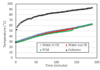
Fig. 2. The HE and the collector temperature in the heating process with solar radiation was 1393.8  $W/m^2$  and the water flow rate was 4 lpm
