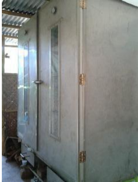
Figure 4. Oven for Drying Simplisia
