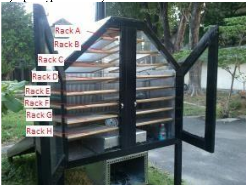
Figure 7. Racks Position in the Solar Dryer Prototype
