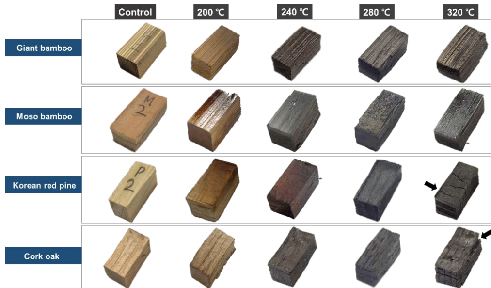
Fig. 1. Appearances of the carbonized samples at different temperatures. Black arrow indicates crack in Korean red pine and split in cork oak
