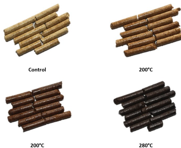
Figure 2. Visual changes of betung bamboo pellets after torrefaction at different temperatures for 50 min.
