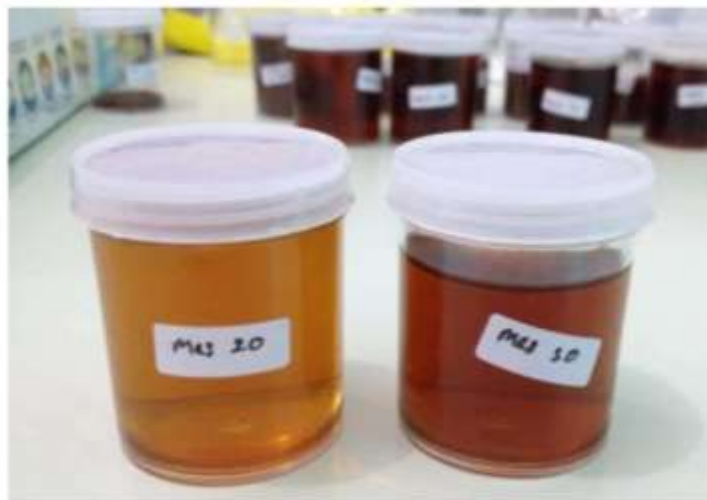
Figure 1. The result of extraction solution for mesh 20 and mesh 30 (particle size of 841 \mu\text{m} and 595 \mu\text{m} ).
