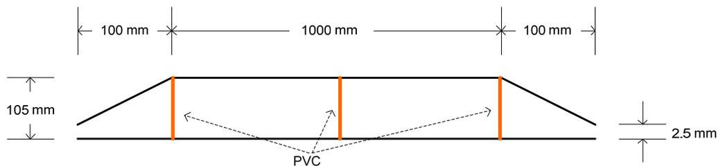
Figure-4. Side view of the TEM cell diagram.
