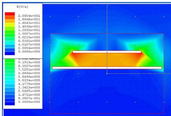
Figure-5. Field plot of designed strip line.
