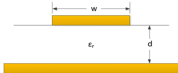
Figure-3. Cross section of strip line geometry.
