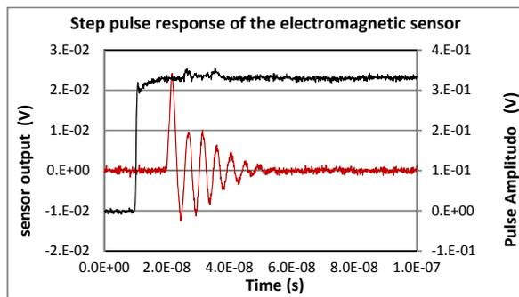
Figure-6. Step pulse response of the Log-spiral sensor.
