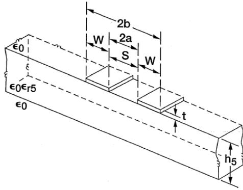
Figure-1. CPS schematic on a dielectric substrate of finite thickness [13].
