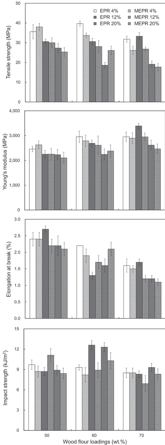
**Fig. 2.** Effect of the impact modifier addition in the presence of MAH and DCP on the tensile properties and impact strength of WF-PP composites with various WF loading. (Note: MAH and DOP content; 1.5 and 0.5 wt%).
