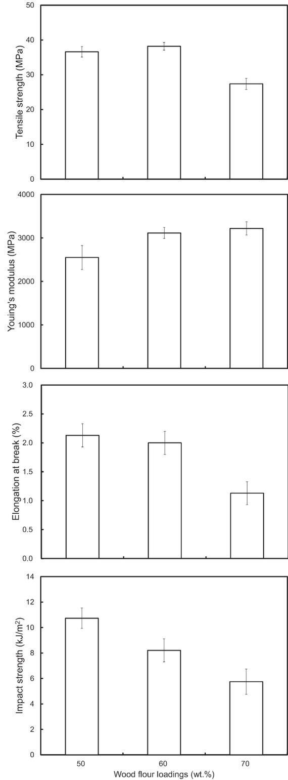
**Fig. 3.** Effect of the addition of EPR, MAPP, and PM on the tensile properties and impact strength of WF-PP composites with different WF loadings. (Note: EPR, MAPP, and PM content; 4.3, 2.5, and 0.2 wt%).
