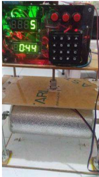
Figure 2. Display of RPM and Time on seven segments.
