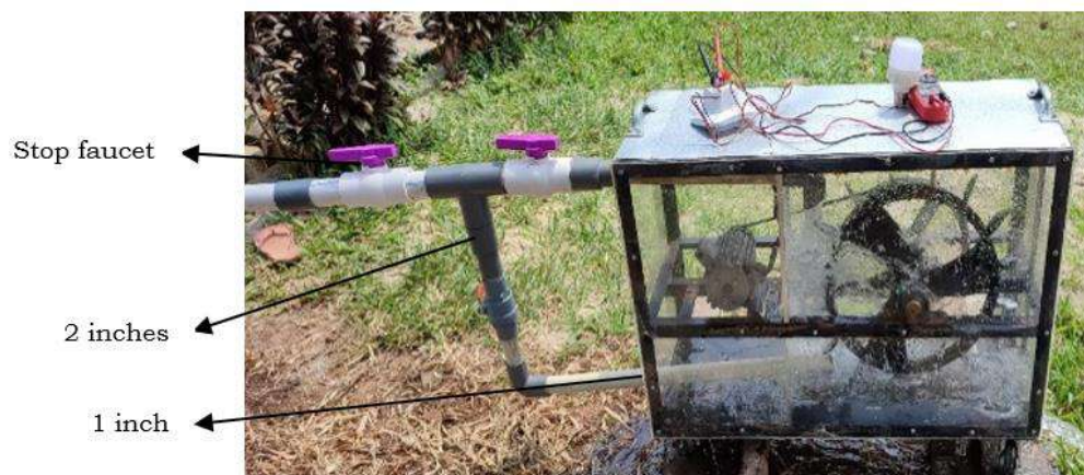
Figure 6. Penstock (PVC Pipe)
