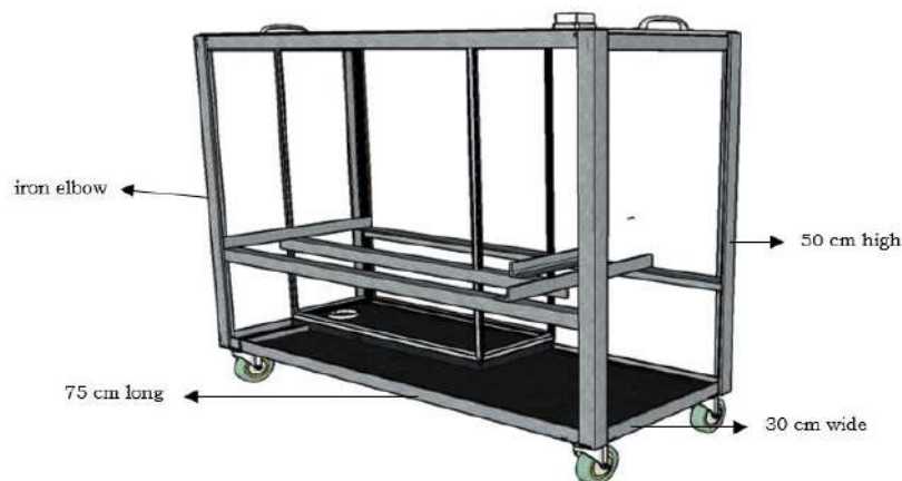
Figure 1. Nano-hydro generator box.
