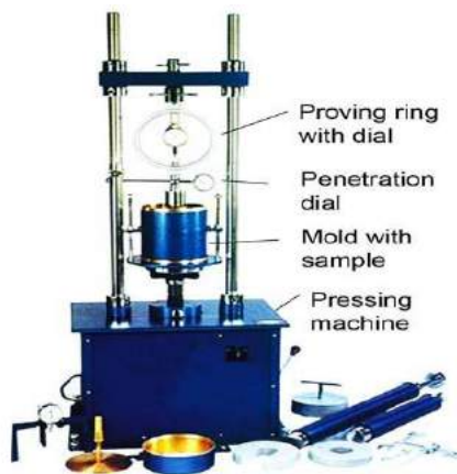
Fig. 2: CBR Test Equipment Source: [34]
