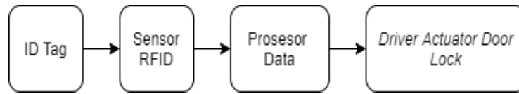
Figure 1. The RFID concept for electronic locking system
