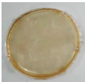
Fig. 5. PIM membrane containing co-EDVB 4% as a carrier
