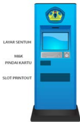
Figure 1. Hardware Kiosk Case Design
