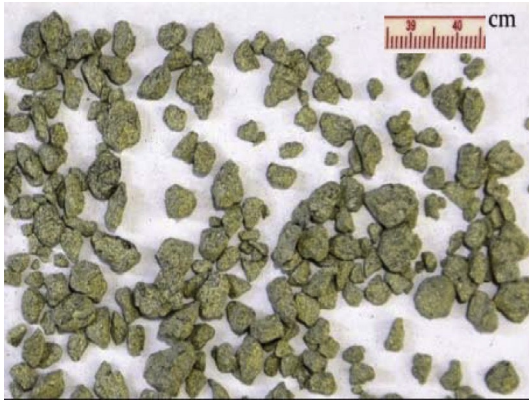
Fig. 1. The form of granular BRA modifier binder (pellets).
