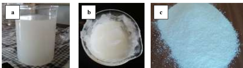
Figure 3. The image of nanocellulose in a form of (a) colloid, (b) gel and (c) powder
