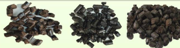
a. Non-torrefied Pellets b. Torrefaction pellets use electric furnaces c. Torrefaction pellets use COMB reaktor
