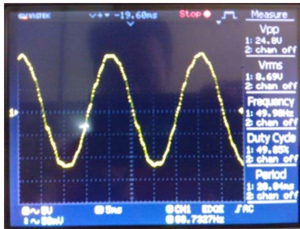
Figure-15. Output voltage when no load condition.
