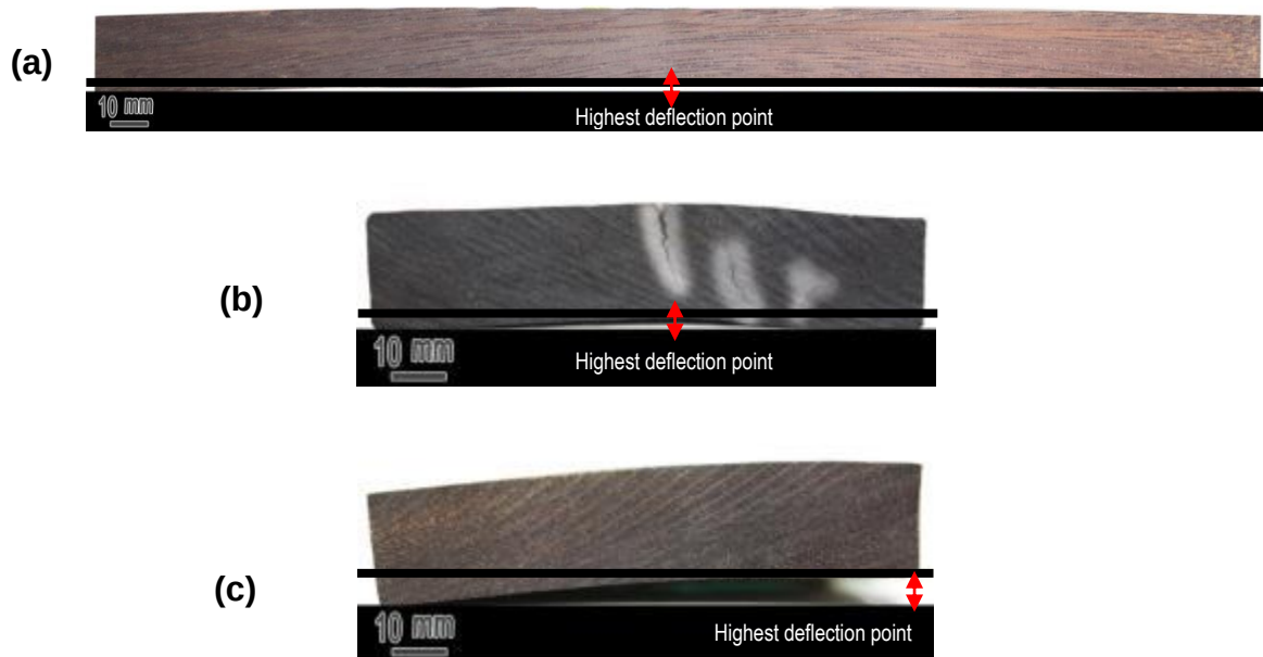
Fig. 3. Measurement of warps: (a) bow, (b) cup, and (c) twist
