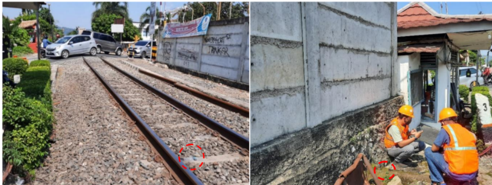
Figure 3. Accelerometer sensors were located at sleeper on left picture and another one on the ground.
