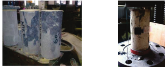
Fig. 4. Compression failure type of specimens with superplasticizer V
