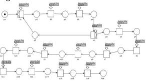
**Figure 5.** Petri Net Service System for Payment of Annual Types of Vehicle Taxes After Repair
