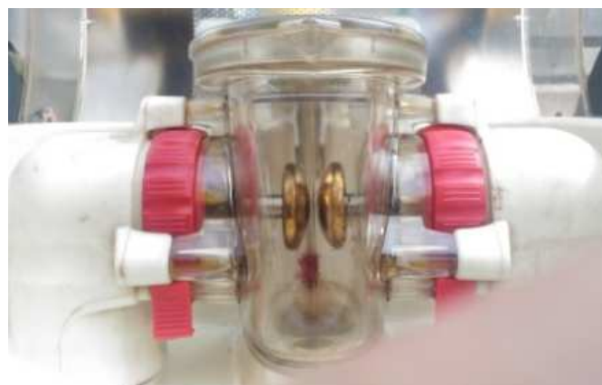
Fig. 7. The breakdown voltage test cup
