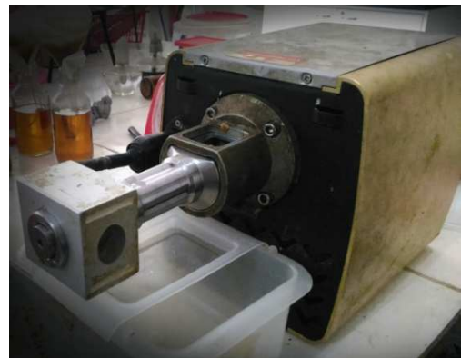
Fig. 1. Pressure machine Newtest is used to produce crude rubber seed oil (CRSO).
