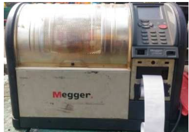
Fig. 6. Megger OTS 80AF used to test the RSO breakdown voltage
